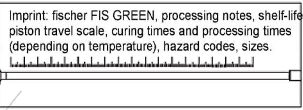
Imprint: fischer FIS GREEN, processing notes, shelf-life, piston travel scale, curing times and processing times (depending on temperature), hazard codes, sizes.
