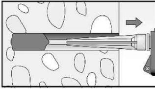
Inject the mortar from the back of the hole towards the front and slowly withdraw the mixing nozzle step by step with each trigger pull. Avoid bubbles. Fill holes approximately 2/3 full, to ensure that the annular gap between the rebar and the concrete will be completely filled with adhesive over the entire embedment length.
