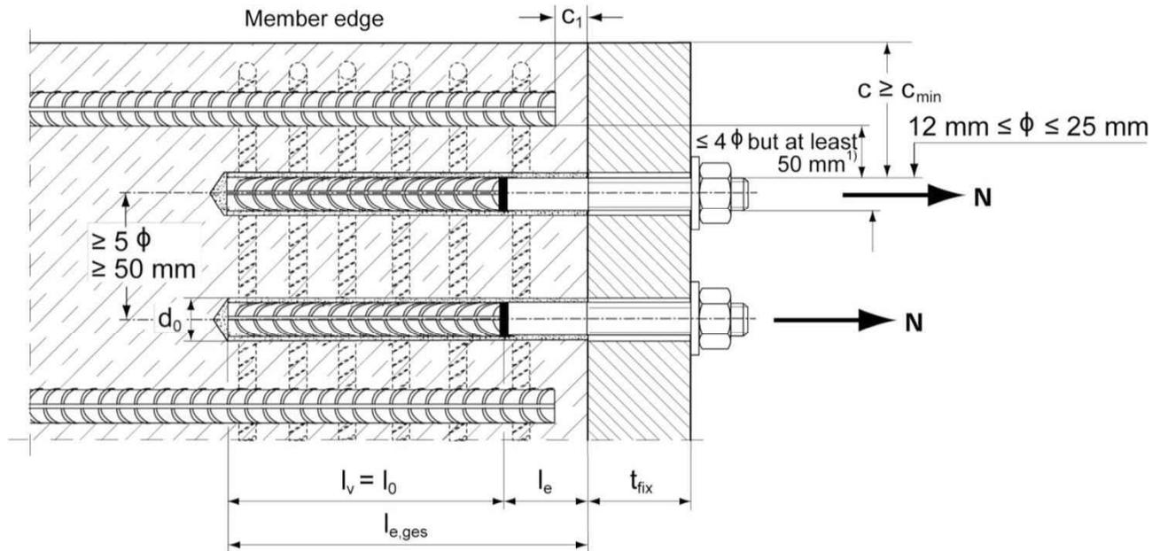
1) If the clear distance between lapped bars exceeds  $4\phi$  but at least 50 mm then the lap length shall be increased by the difference between the clear bar distance and  $4\phi$  but at least 50 mm.
