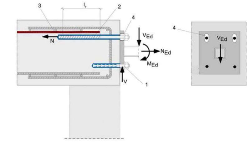
The required transverse reinforcement acc. to EN 1992-1-1:2011 is not shown in the figures. **The fischer rebar anchor may be only used for axial tensile force.** The tensile force must be transferred by lap to the existing reinforcement of the building. The transfer of the shear force has to be ensured by suitable measure, e.g. by means of shear force or anchors with European Technical Assessment (ETA).
