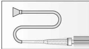
Assemble mixing nozzle FIS MR Plus or FIS UMR, extension tube and appropriate injection adapter (see table B 6.2)
