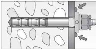
After inserting the pre-assembled anchor rod, excess mortar must be emerged around the Fischer filling disc (minimum on one point).
