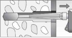
Fill approximately 2/3 of the drill hole incl. fixture with mortar. Always begin from the bottom of the hole and avoid bubbles.
