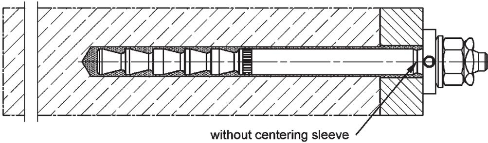
Push through installation without shear force sleeve, FHB dyn (annular gap filled with mortar)
