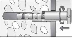
Push the pre-assembled Fischer anchor rod (with shear force sleeve, centering sleeve, Fischer filling disc, spherical washer, hexagon nut and lock nut) into the drill hole until the Fischer filling disc is in full contact with the surface, turning it slightly while doing so.
