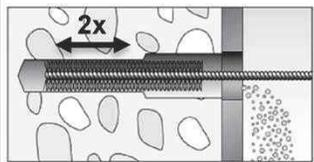
Brush the drill hole 2 of the borehole twice with a steel brush.
