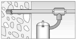
Use a suitable dust extraction system, e.g. fischer FVC 35 M or a comparable dust extraction system with equivalent performance data.
