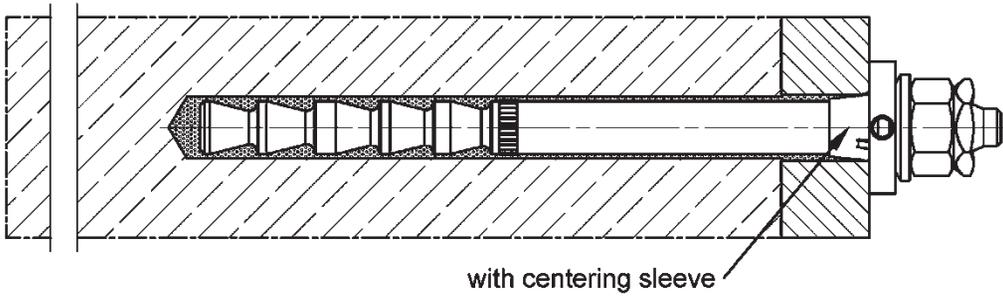
Push through installation with shear force sleeve, FHB dyn V (annular gap filled with mortar)
