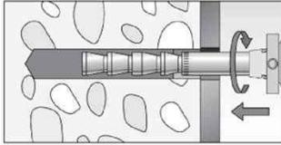
Push the pre-assembled Fischer anchor rod (with centering sleeve, Fischer filling disc, spherical washer, hexagon nut and lock nut) into the drill hole until the Fischer filling disc is in full contact with the surface, turning it slightly while doing so.
