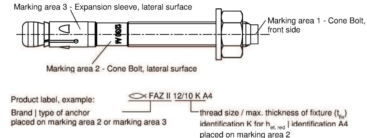
**Table A2:** Letter-code on marking area 1 and maximum thickness of fixture  $t_{fix}$ :
