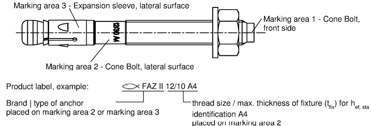
**Table A1:** Letter-code on marking area 1 and maximum thickness of fixture  $t_{fix}$ :
