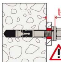
10: Correctly installed fastener
