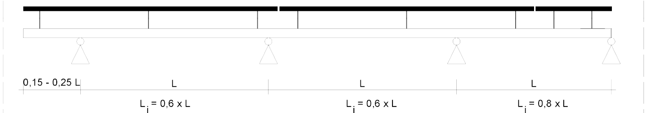
Figure 4: Equivalent support spacing
