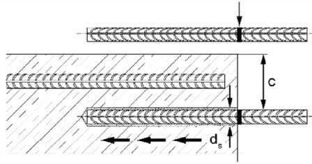
Before use, make asure that the rebar or the fischer rebar anchor is dry and free of oil or other residue. Mark the embedment depth  $l_v$  resp.  $l_{e,ges}$  (e.g. with tape) Insert rebar in borehole, to verify drill hole depth and setting depth  $l_v$  resp.  $l_{e,ges}$
