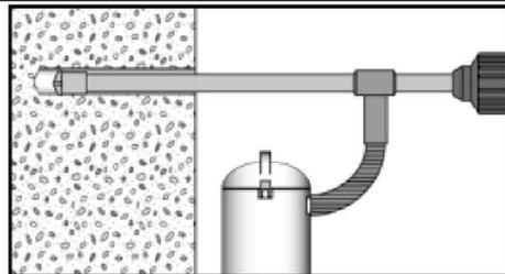
Use a suitable dust extraction system, e. g. fischer FVC 35 M or a comparable dust extraction system with equivalent performance data. Drill the hole with hollow drill bit. The dust extraction system has to extract the drill dust nonstop during the drilling process and must be adjusted to maximum power. No further drill hole cleaning necessary
