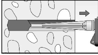
Inject the mortar from the back of the hole towards the front and slowly withdraw the mixing nozzle step by step with each trigger pull. Avoid bubbles.
