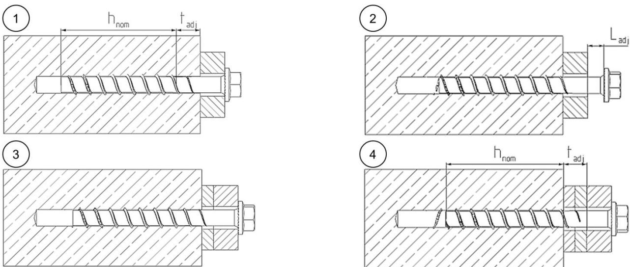
It is permissible to untighten the screw up to two times for adjustment purposes.
