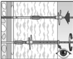
4. Press the anchor with the screw plate tight against the surface of the insulation material, then start screwing-in the anchor. Setting is finished when the surface of the ring is flush with the surface of the insulation material.
