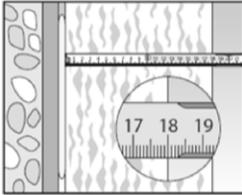
1. Measure insulation thickness  $h_D$
