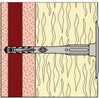
4. Correctly installed anchor.
