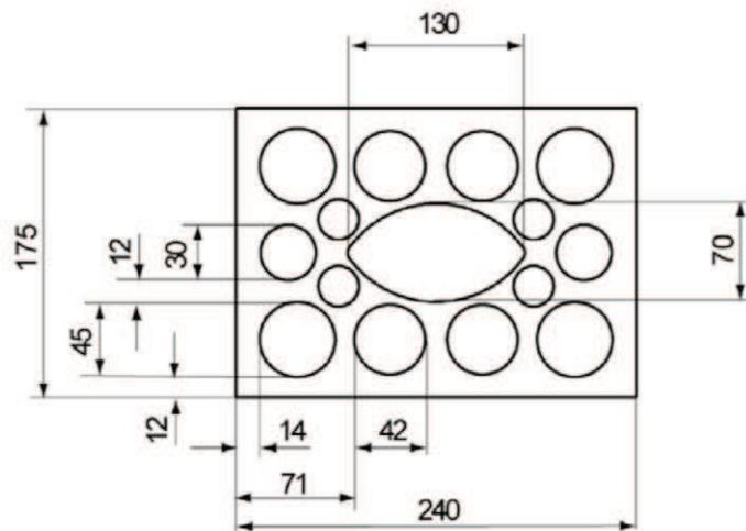
**Table C32: Installation parameters for threaded rod with perforated sleeve
