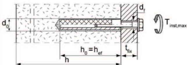
Threaded rods and internal threaded anchors FIS E without perforated sleeve FIS H K; installation in autoclaved aerated concrete (installation with special conic drill bit PBB)
