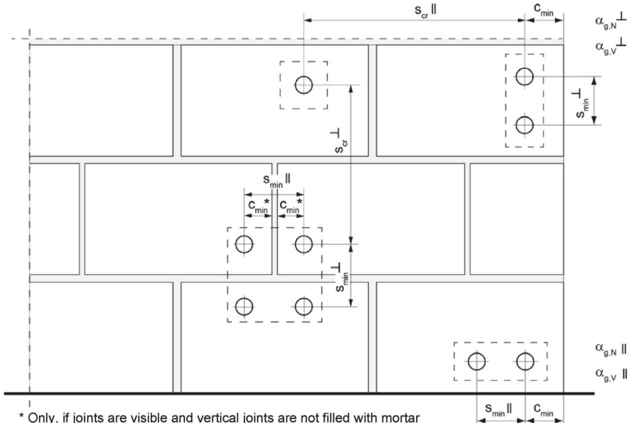
$s_{min} \parallel$  = Minimum spacing parallel to bed joint
