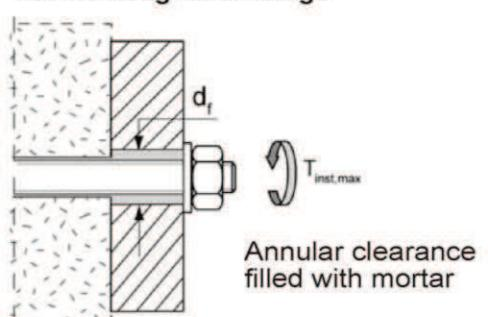
Internal threaded anchors FIS E without perforated sleeve FIS H K; installation in solid brick masonry and autoclaved aerated concrete
