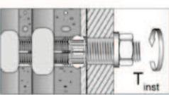
Mounting the fixture.<br>$T_{inst,max}$ see parameter of brick.                                                                                                   |
