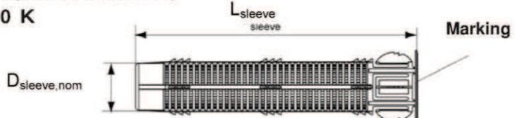
**Table B4: Installation parameters for threaded rods with perforated sleeves (push through anchorage)**
