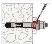
9: The gap between anchor and fixture (annular gap) must be filled with mortar (compressive strength  $\geq 50 \text{ N/mm}^2$  e.g. fischer FIS HB, FIS V Plus, FIS EM Plus or FIS SB) via the fillable conical washer.
