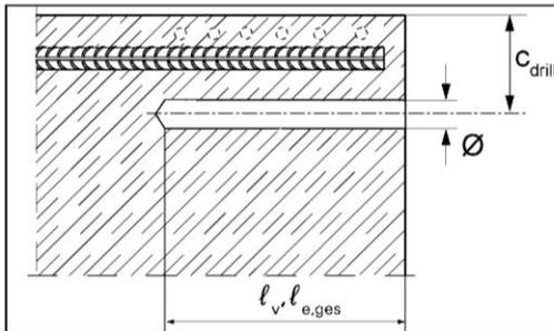
Measure and control concrete cover  $c$
