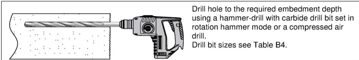
Drill hole to the required embedment depth using a hammer-drill with carbide drill bit set in rotation hammer mode or a compressed air drill.
