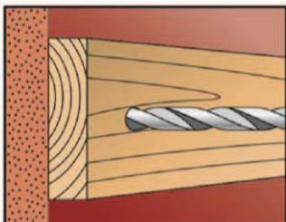
1. Drill the bore hole Ø 8 mm (SXR 8) and Ø 10 mm (SXR 10 / SXRL 10) using the drill method described in the corresponding annex.
