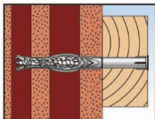
5. Correctly installed anchor in hollow masonry.
