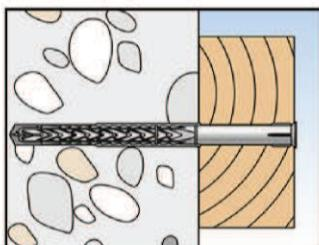
6. Correctly installed anchor in concrete.
