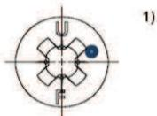
1) Additional marking for the special screw, stainless steel version: „A4“.
