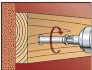
4. The screw is screwed-in until the head of the screw touches the sleeve.
