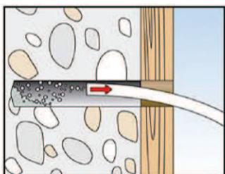
2. Remove dust from borehole.
