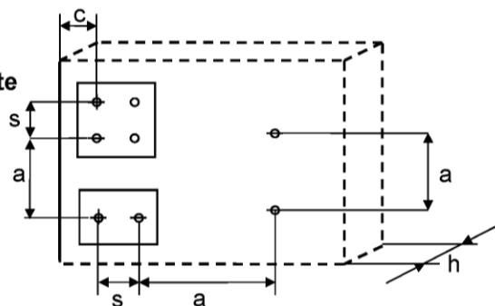
**Scheme of distance and spacing in concrete****fischer frame fixing SXR / SXRL****Intended use**
