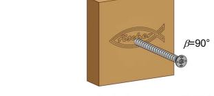
Figure D5.1: Screw arrangement in the plane surface of WBP (figure not to scale)
