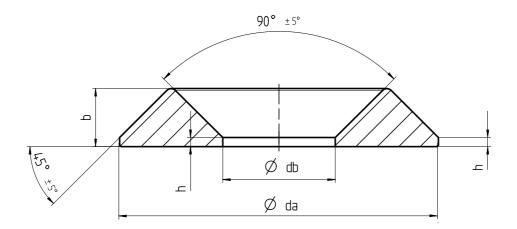
Washer for Power-Fast and construction screws
