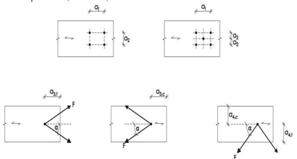
Definition of spacing, end and edge distances in the edge surface unless otherwise specified in the technical specification (ETA or hEN) for the cross laminated timber.
