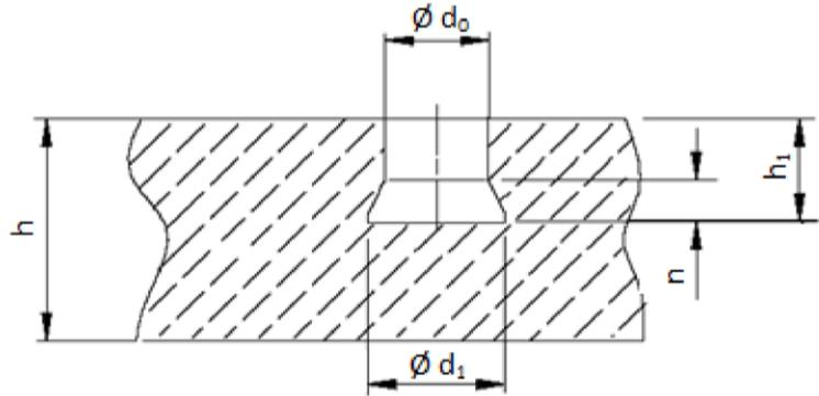
**Table B3: Drill bit assignment and dimensions of drill bit and drill hole [mm]**
