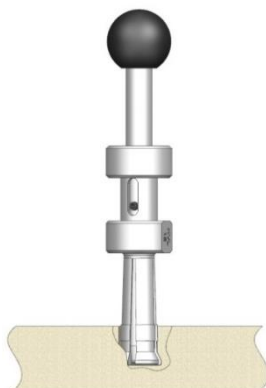
HVL-T (Undercut minimum volume gauge)
