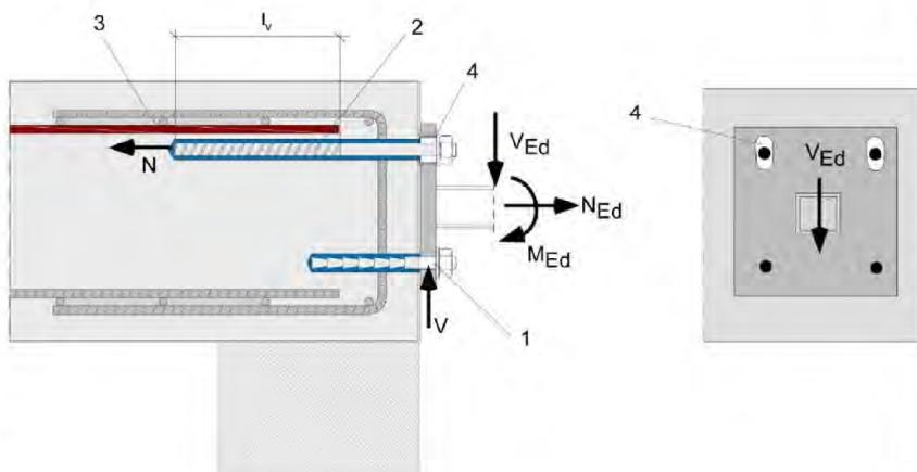
The required transverse reinforcement acc. to EN 1992-1-1:2004+AC:2010 is not shown in the figures. **The fischer rebar anchor FRA may be only used for axial tensile force.** The tensile force must be transferred by lap to the existing reinforcement of the building. The transfer of the shear force has to be ensured by suitable measure, e.g. by means of shear force or anchors with European Technical Assessment (ETA)
