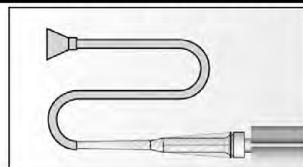
Assemble static mixer, extension tube and appropriate injection adapter (see table B6.2)
