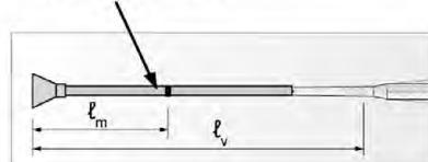
Mark the required mortar level  $l_m$  and embedment depth  $l_v$  resp.  $l_{e,ges}$  with tape or marker on the injection extension tube.
