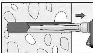
Inject the mortar from the back of the hole towards the front and slowly withdraw the mixing nozzle step by step with each trigger pull.
