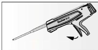
After injecting, release the dispenser. This will prevent further mortar discharge from static mixer.
