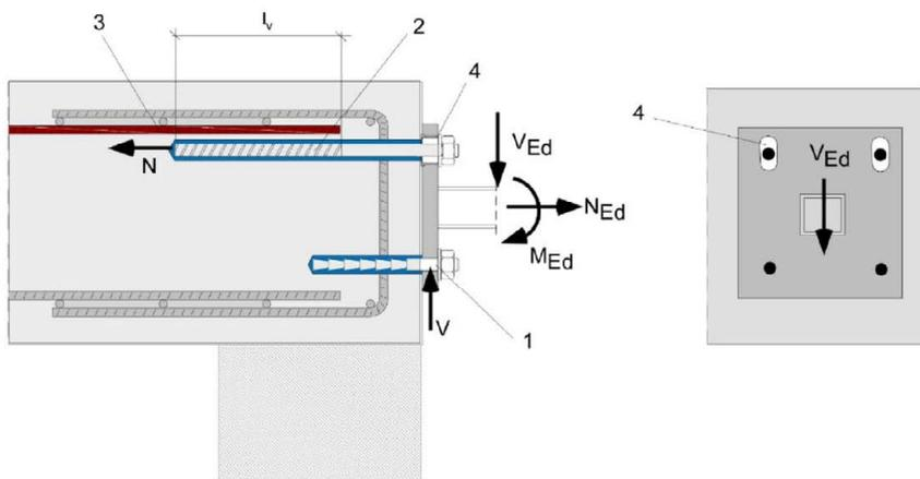
The required transverse reinforcement acc. to EN 1992-1-1:2011 is not shown in the figures. **The fischer rebar anchor FRA may be only used for axial tensile force.** The tensile force must be transferred by lap to the existing reinforcement of the building. The transfer of the shear force has to be ensured by suitable measure, e.g. by means of shear force or anchors with European Technical Assessment (ETA).
