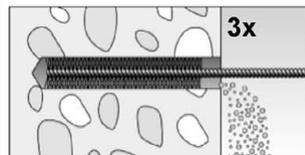
Brush drill hole three times; for drill hole diameters  $d_0 \geq 30$  mm attach brush to a power tool and brush hole with a speed of max. 550 revolutions per minute. For deep holes a brush extension is mandatory. Use suitable brushes (see **Table B6.2**).
