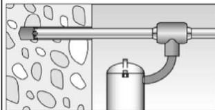
Use a suitable dust extraction system, e. g. fischer FVC 35 M or a comparable dust extraction system with equivalent performance data. Drill the hole with hollow drill bit. The dust extraction system has to extract the drill dust nonstop during the drilling process and must be adjusted to maximum power. No further drill hole cleaning necessary.
