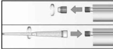
Twist off the sealing cap
