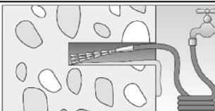
Flush the drill hole, until clear water emerges from the drill hole.
