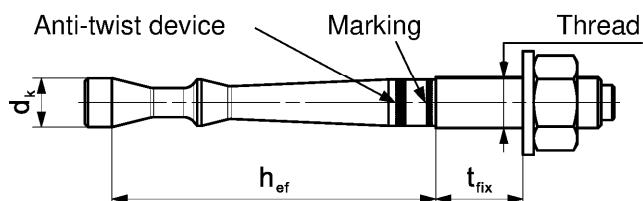
**Marking:** work symbol, thread diameter, embedment depth e.g.:
