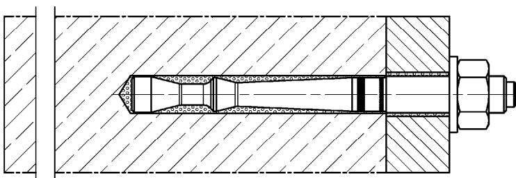
**Pre-positioned or push through installation** with subsequently injected fischer filling disc
