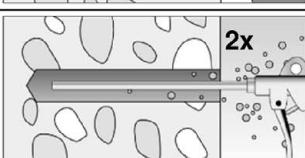
Blow out the drill hole twice, using oil-free compressed air ( $p \geq 6$  bar)
