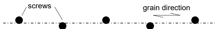
Figure D7.1: Staggered arrangement of the screws parallel to the grain direction (figure not to scale)
