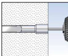
3: Turning the internal thread bolt with the hexagon (approximately 15 turnings are required)
