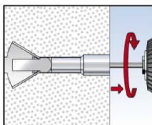
4: By turning the internal thread bolt, the cone is driven into the expansion sleeve. When the optimal expansion is reached, the hexagon is thrown out of the socket. **The turning of the internal thread bolt until the hexagon is thrown out of the socket is compulsory** if tightening is impossible the anchor cannot be loaded
