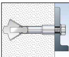
5a: Optional tightening the fastener with a torque  $T_{\max} \leq 3$  Nm. The anchor could be pulled against the fixture depending on the compressive strength of the AAC.
