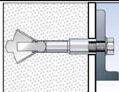
5b: If the anchor cannot support against the fixture (with cover layer) no installation torque may be applied ( $T_{max} = 0$ )
