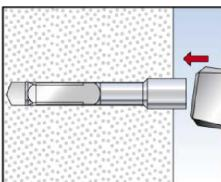
2: Set the fastener until it is flush with the surface of the AAC
