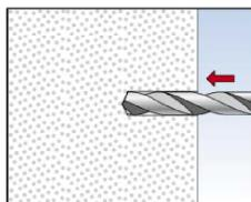
1: Drill the hole. Other methods like punching, to make the hole, are allowed. When the AAC is covered with a hard layer like tiles, the tile has to be drilled with minimum diameter of the head of the internal threaded bolt  $\varnothing$  D
