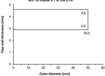
Interpolation between pipe diameters and wall thicknesses for plastic pipes according to clause 2.1 of the ETA in flexible walls, rigid walls and rigid floors - mixed penetration seal
