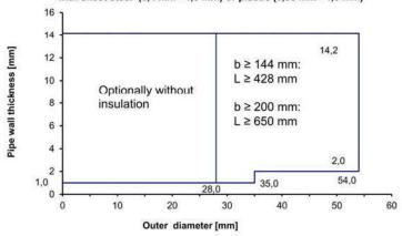
L measured from the surface of the penetration seal (see ANNEX B-1 to C-2 of the ETA).
