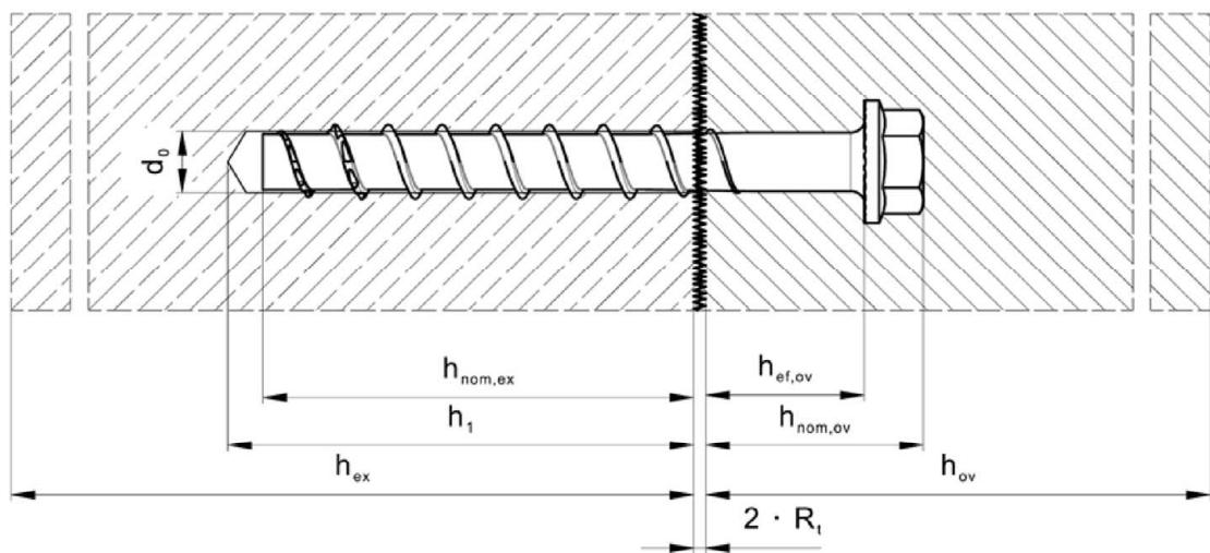
$h_{\text{nom},\text{ex}}$  Overall embedment depth in existing concrete
