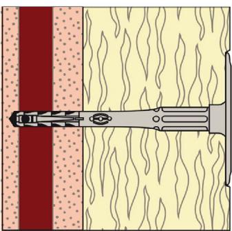
4. Correctly installed anchor.
