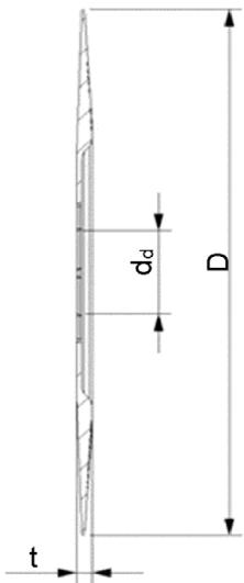
**Table A10.2: Slip-on plate, dimensions and material**
