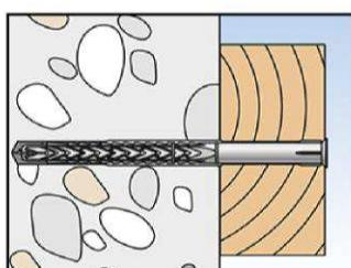
6. Correctly installed anchor in concrete.
