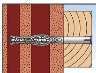
5. Correctly installed anchor in hollow masonry.
