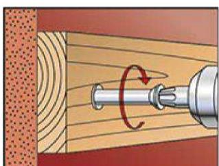
4. The screw is screwed-in until the head of the screw touches the sleeve. The anchor is correctly mounted, when the head of the screw fits tight on the surface and cannot be screwed-in any further.
