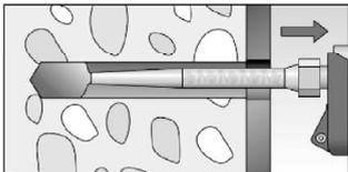
Fill approximately 2/3 of the drill hole incl. fixture with mortar. Always begin from the bottom of the hole and avoid bubbles.
