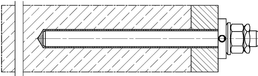
**Push through installation with the necessary components** (annular gap filled with mortar)
