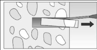
Break the drill core and remove it |
