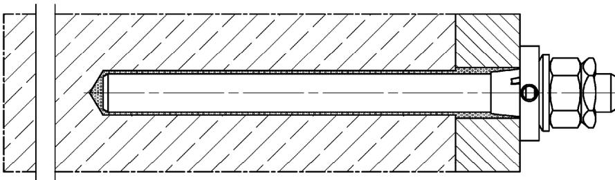
**Push through installation with the necessary components** (annular gap filled with mortar)
