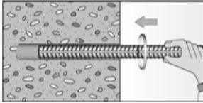
For each installation insert the rebar slowly twisted into the borehole until the embedment mark is at the concrete surface level.
