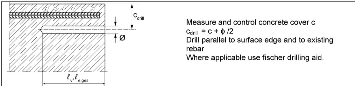
Measure and control concrete cover  $c$
