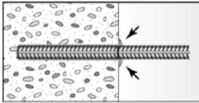
After installing the rebar the annular gap must be completely filled with mortar.
