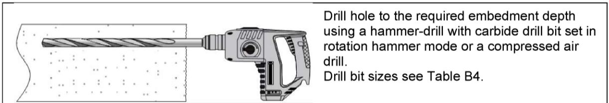
Drill hole to the required embedment depth using a hammer-drill with carbide drill bit set in rotation hammer mode or a compressed air drill.
