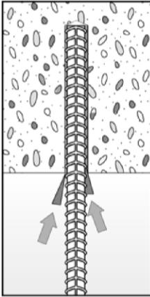
Support the rebar and secure it from falling till mortar started to harden, e.g. using wedges.
