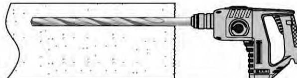
Drill hole to the required embedment depth using a hammer-drill with carbide drill bit set in rotation hammer mode, a pneumatic drill or a diamond drill in drilling mode.
