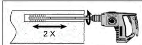
Fix an adequate steel brush with an extension into a drilling machine and brush the bore hole two times
