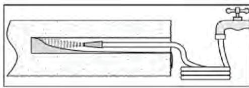
Flush the bore hole until the water comes clear
