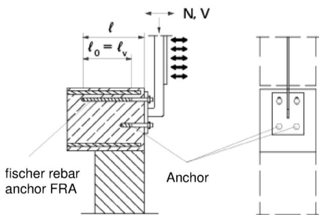
**Figure A7:** Lap of the anchoring of guardrail posts.
