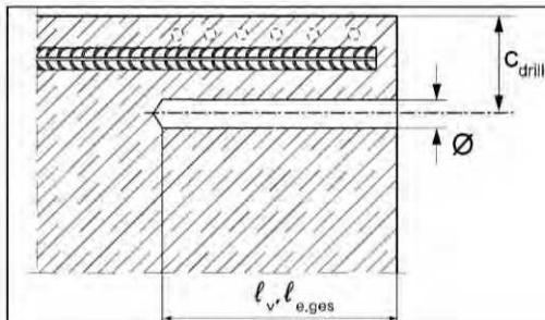
Measure and control concrete cover  $c$
