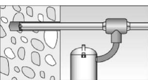
Use a suitable dust extraction system, e.g. fischer FVC 35 M or a comparable dust extraction system with equivalent performance data.
