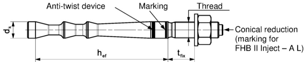
**Marking:** work symbol, size of anchor, setting depth. e.g.: M10x95
