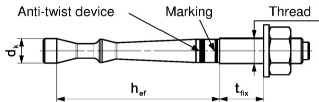
**Marking:** work symbol, size of anchor, setting depth. e.g.: M10x75
