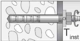
Tighten the hexagon nut with installation torque  $T_{inst}$  (see **Table B5.1**).
