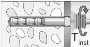
Tighten the hexagon nut with installation torque  $T_{inst}$  (see **Table B6.1**).
