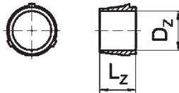
Conical washer / fischer filling disc:
