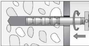
Push the pre-assembled Fischer anchor rod (with washer and hexagon nut) into the drill hole until the Fischer filling disc is in full contact with the surface, turning it slightly while doing so.
