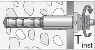
Tighten the hexagon nut with installation torque  $T_{inst}$  (see **Table B7.1**).
