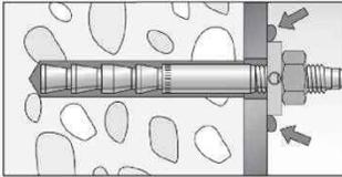
After inserting the pre-assembled anchor rod, excess mortar has to emerge under the washer.
