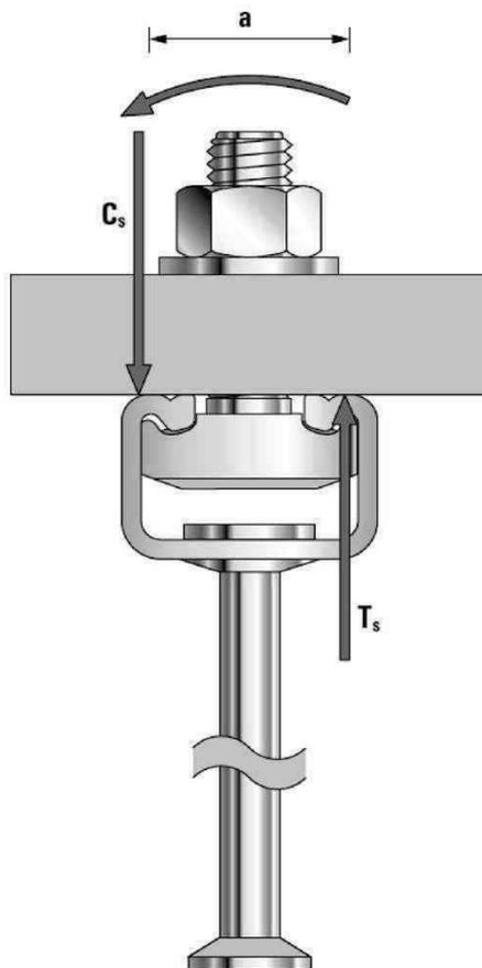
$$M^{0}_{RK,s} \leq 0,5 \cdot N^{0}_{RK,s,l} \cdot a \quad (N^{0}_{RK,s,l} \text{ according to Table C1.1})$$
