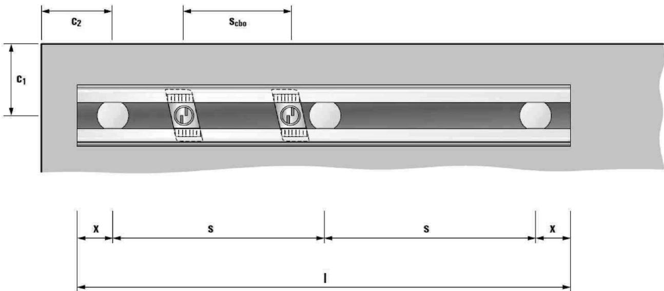
**Table B3.2:** Minimum spacing for channel bolts
