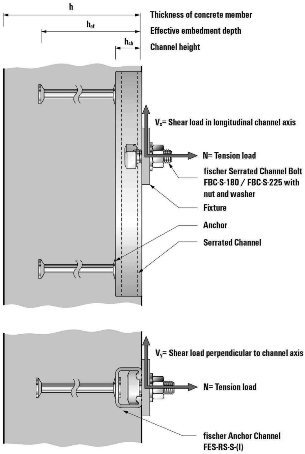
**fischer Serrated Anchor Channel InnoLock FES-RS-S with fischer Serrated Channel Bolts FBC-S**
