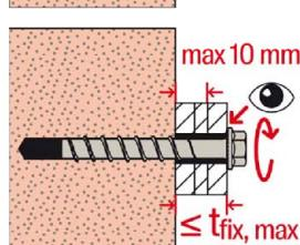
The maximum shimming  $t_{adj} = 10\text{mm}$  must not be exceeded.
