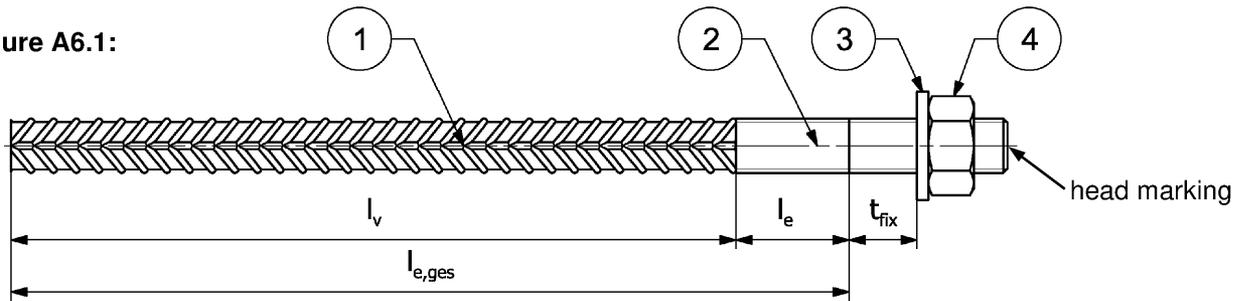
Head marking e.g.:
