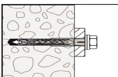
5. Correctly installed anchor in concrete.
