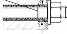
Anchor rod Push through anchor (annular gap filled with mortar)
