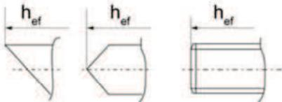
Alternative point geometry threaded rod RGM
