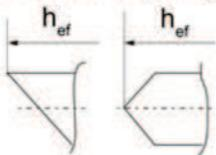
Alternative head geometry threaded rod FIS A and RGM
