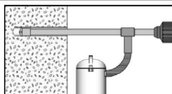
Drill the hole to the required embedment depth using a hammer drill with hollow drill bit in rotation hammer mode.
