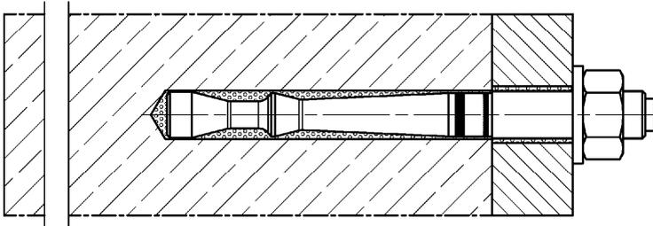
Pre-positioned or push through installation with subsequently injected fischer filling disc (annular gap filled with mortar)
