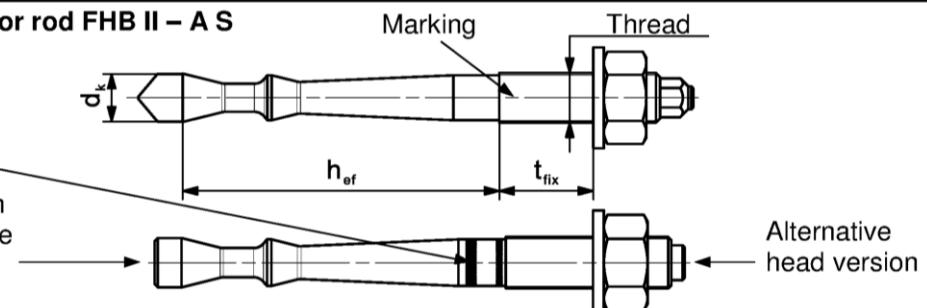
**Marking:** work symbol, size of anchor, setting depth. e.g.: M10x75
