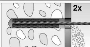
Brush the drill hole twice with steel brush.
