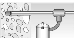
Use a suitable dust extraction system, e. g. fischer FVC 35 M or a comparable
