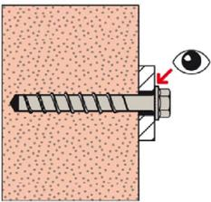
After installation further turning of the screw must not be possible. The maximum installation torque (max  $T_{inst}$  according to Annex C) must not be exceeded during checking.
