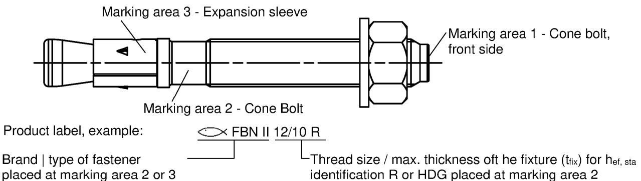
**Table A2.1:** Letter-code on marking area 1 and maximum thickness of fixture  $t_{fix}$  [mm]:
