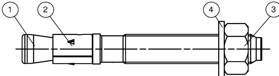
Cone bolt manufactured by turning:
