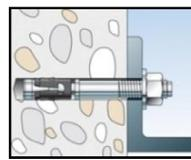
5: Installed fastener
