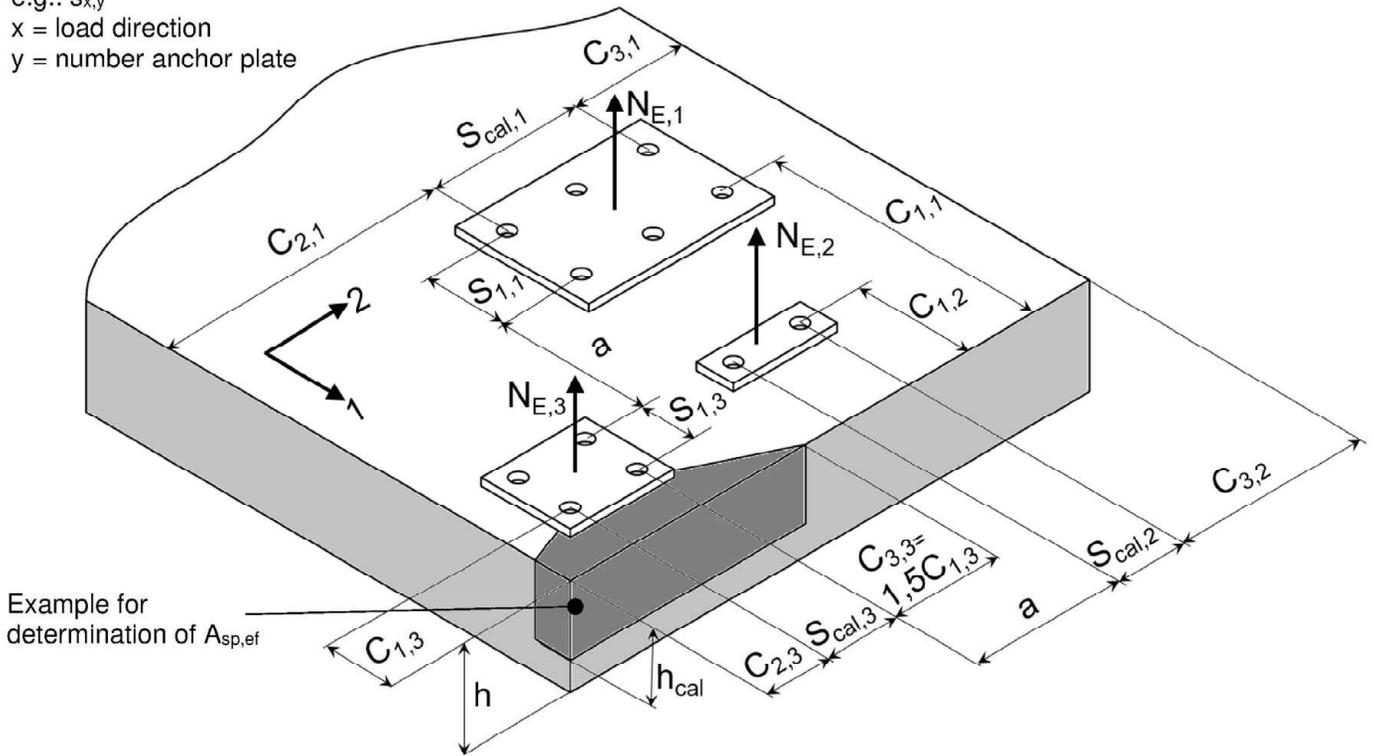
Example for different anchor plates: For considering all free edges the direction 1 and 2 must be swapped.
