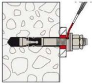
9: The gap between anchor and fixture (annular gap) must be filled with mortar (compressive strength  $\geq 50 \text{ N/mm}^2$  e.g. fischer FIS HB, FIS V Plus, FIS EM Plus or FIS SB) via the fillable conical washer.
