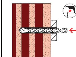
1. Drill the bore hole as per Table B2.1 using the drilling method described in the corresponding Annex C.
