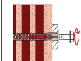
4. The screw is screwed-in until the head of the screw touches the sleeve. The anchor is correctly installed, if the head of the screw fits tight on the surface and nor the anchor sleeve neither the screw cannot be turned-in any further.
